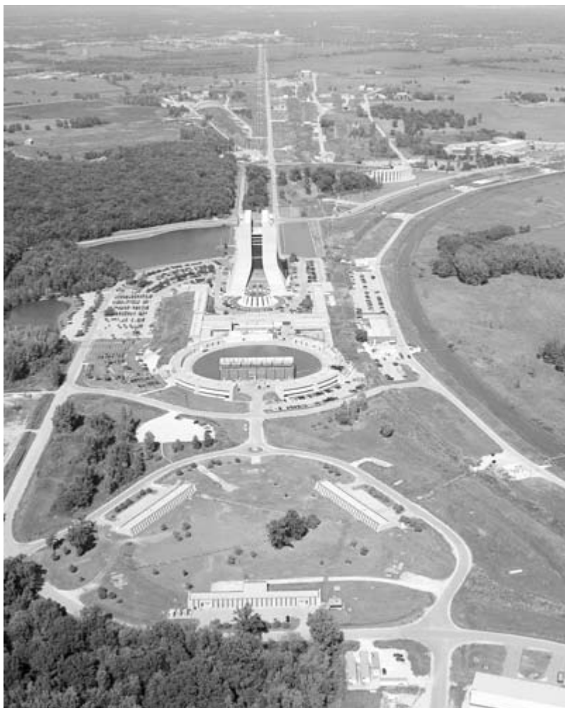
12.3 Aerial view of Fermilab showing the High-Rise (Wilson Hall), the Booster ring below, in the center of the photo, and the larger rounded triangle of the antiproton source, 1999. (Courtesy of FNAL Visual Media Services.)
